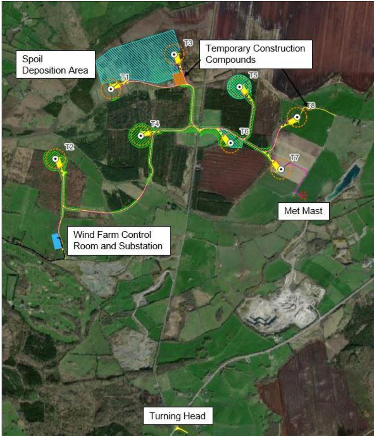
Figure 10.1: Aerial Photograph Showing Location of Turbines 1–8 & Associated Infrastructure
