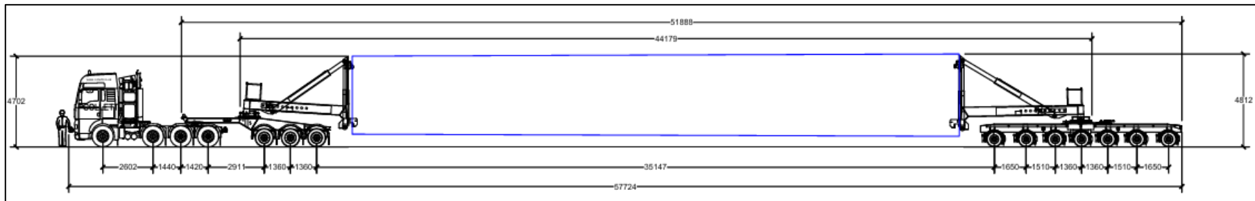
Figure 14.3: Typical Tower Section Transport
